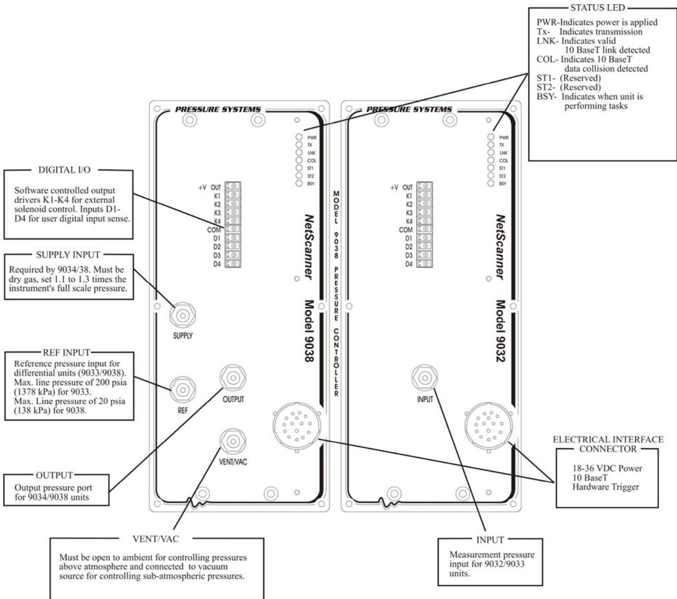
This example depicts the electrical/pneumatic connection and required cables and support equipment necessary to interface a 9038 to a host computer. Shop air may be used for the supply if it is free of moisture, oil and contaminants.
