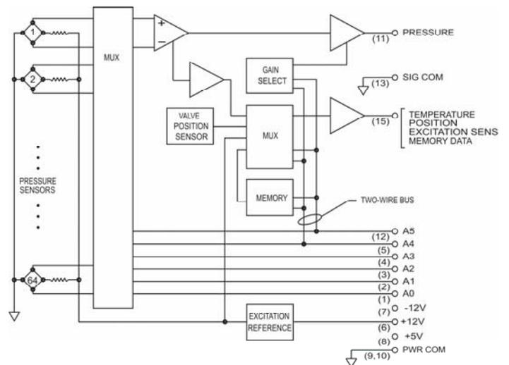
Another advanced feature is the ability to derange the ESP scanner upon command. This alters the gain on the amplifier to derange the scanner by a factor of three, enabling additional windtunnel tests to be conducted without re-instrumenting the model with lower range ESP scanners. To optimize the accuracy of the DTC scanner at the highest gain, the optional dual range calibration is recommended.
