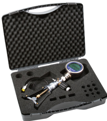
Basic version incl. pneumatic pressure generation
